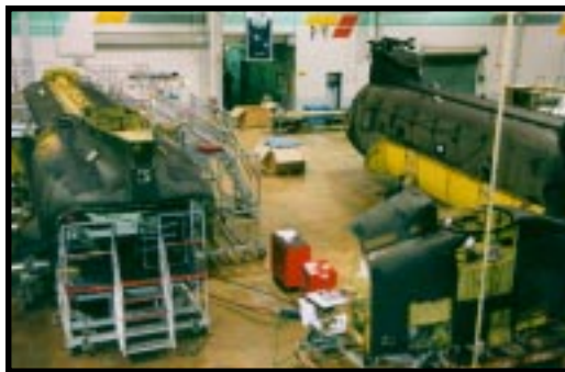
CH-47F prototypes are well on their way through the tear-down process as the first step in the upgrade program. □
