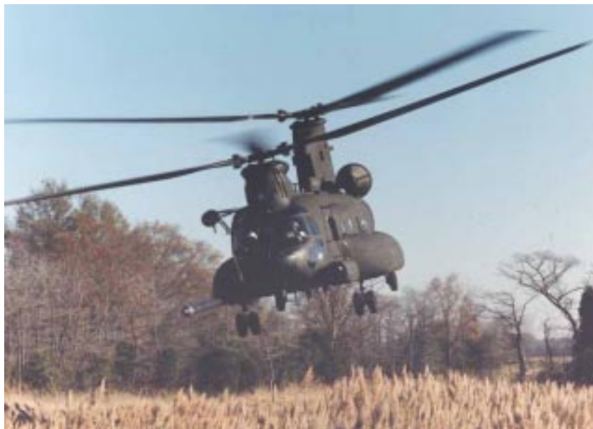
Comin' at Ya. The MH-47E Special Operations Chinook doing what it does best, flying nap-of-the-earth at high speed. With deliveries completed in 1994, the U.S. Army's MH-47Es remain among the most advanced helicopters flying today. Among the distinguishing features in this photo are the in-flight refueling boom, rescue hoist, chin-mounted forward-looking infrared turret and terrain-following, terrain-avoidance radar. □
