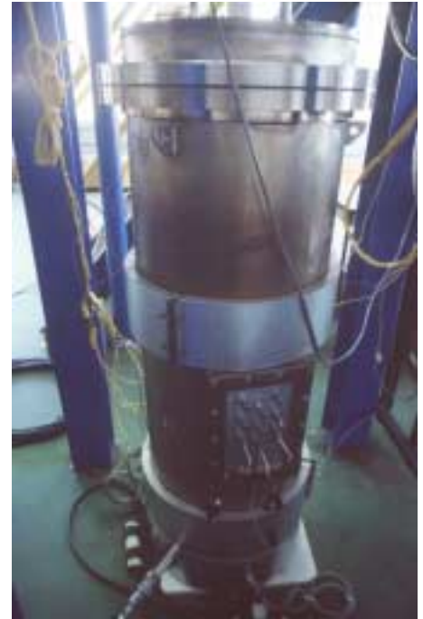
Half-height mockup of the Irradiated Fuel Storage Facility Fuel Canning Station showing instrument port for monitoring temperature and pressure during drying.
