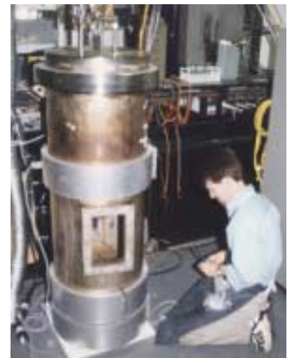
Warm vacuum drying test being prepared for mock fuels.
