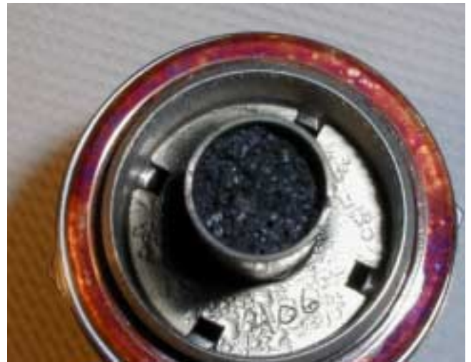
Unirradiated metallic uranium fuel corrosion: Test coupon completely corroded after 77 days in unsaturated test conditions at 90° C. Work performed at Argonne National Laboratory-East.
