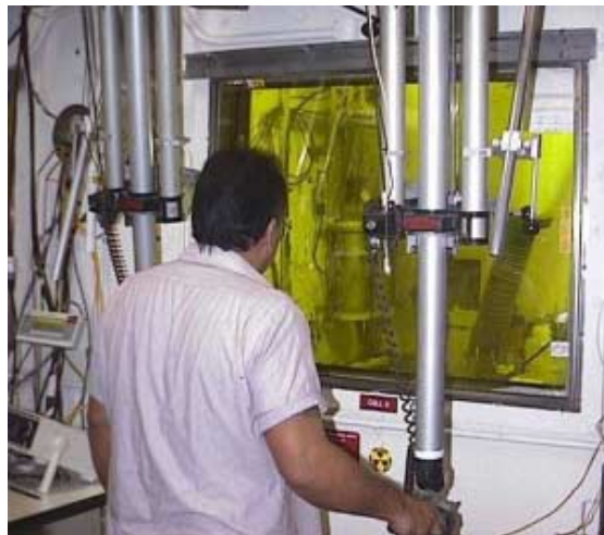
Hot cells are used to manipulate radioactive samples. Hot cell shown is at Pacific Northwest National Laboratory.
