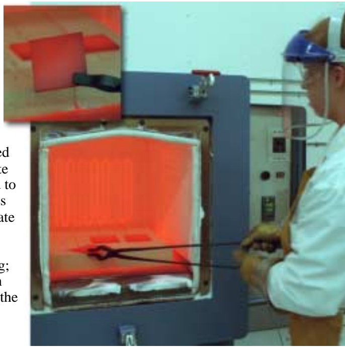
Removing 316L stainless steel coupons after heat sensitizing heat treatment.
