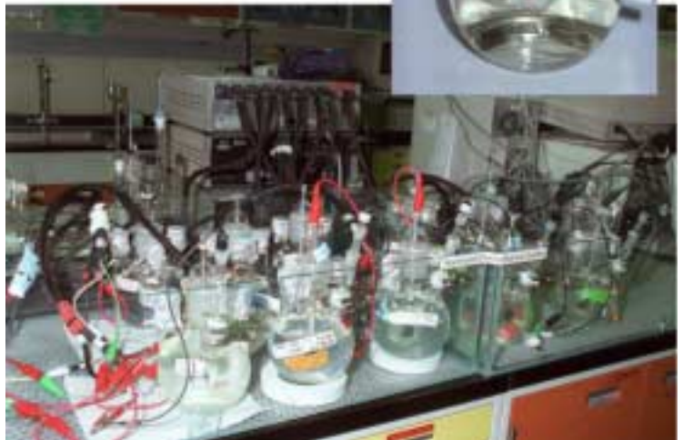
Test cells are used to expose metal coupon to corrosive fluid, and measure the corrosion (degradation) rate. (microbiologically influenced corrosion)
