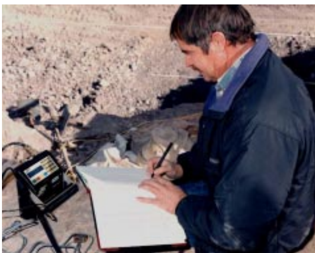
Monitoring water table fluctuations at a borehole
