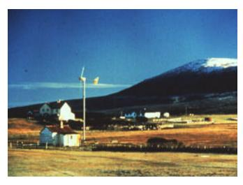
Usually a tower between 80 and 120 feet in height is supplied with the wind turbine. Towers of this height raise the turbine above turbulence generated by obstacles (such as buildings and trees) on the ground. Also, wind velocity increases with greater altitude, so wind turbine performance improves with height.
