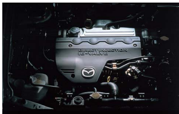
DI-TD (Direct-Injection Turbo Diesel) Engine Exhaust output of water-cooled in-line four cylinder DOHC 16 valve diesel engine: 1,998cc Maximum output: 100ps / 4,000rpm Maximum torque: 22.4kg-m / 2,000rpm
