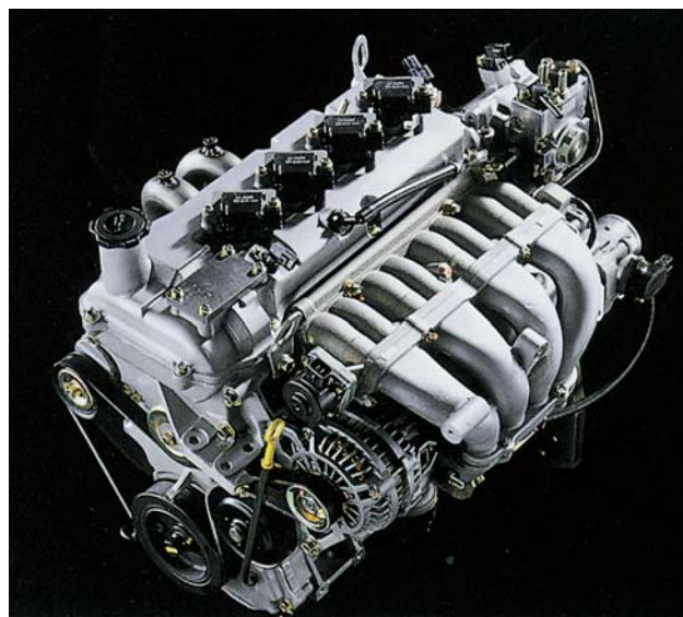
Mazda DIREC-G Exhaust output of water-cooled in-line four cylinder DOHC 16 valve gasoline engine: 1,498cc Maximum output (target value): 77kW (105PS) / 6,000rpm Maximum torque (target value): 105N·m (15.2kg-m) / 3,500rpm
