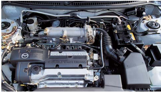
S-VT Engine Maximum output: 96kW (130PS)/7000rpm Maximum torque: 141N·m(14.4kg-m)/4000rpm
